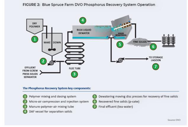
The entire system is semi-automated for continuous operation, only turning off when float valves on the equalization pit determines the need to temporarily stop due to low manure volume. The system restarts operations automatically when more manure is available. Ernie Audet said, "Regular operations and maintenance is a daily walk-through and completion of a monitoring checklist with a morning filling of solid polymer to a feed hopper."
