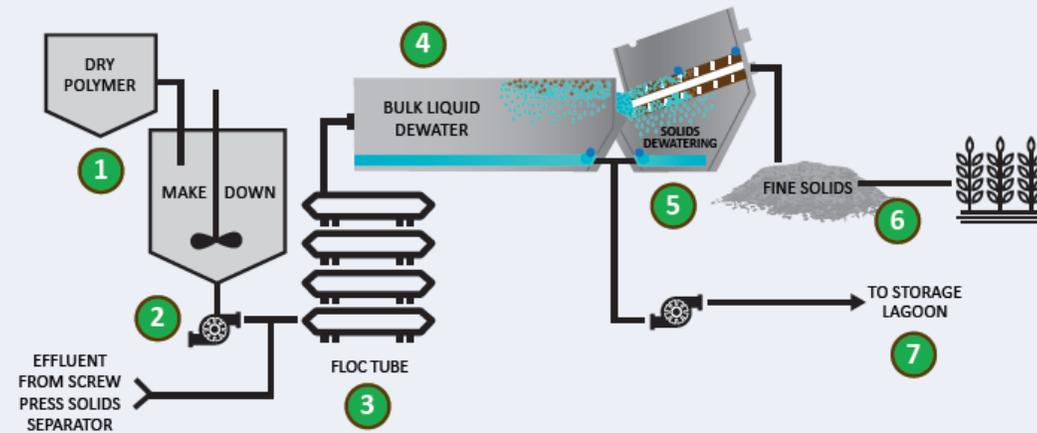
**The Phosphorus Recovery System key components:**
