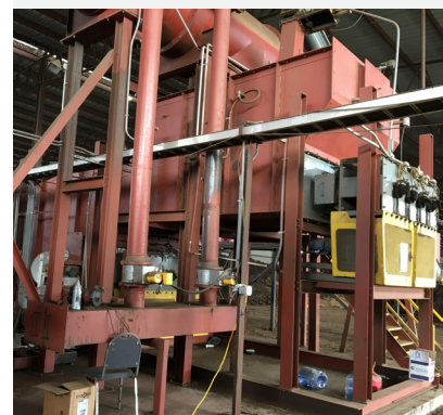
The Coaltec Energy gasification manure dryer.
