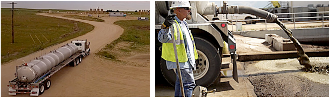
Figure 2. Eight to ten tanker truckloads daily deliver over 100,000 gallon of manure at 15% solids.
