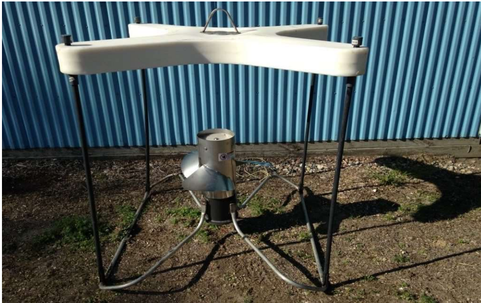
Figure 1. PondLift floating aerator.
