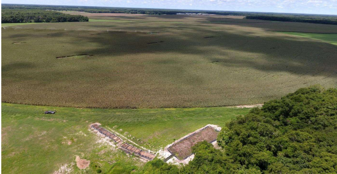
Figure 5. Aerial view of Pivot B with milking barns in the distance and denitrification bioreactor in the foreground. Open patches within the sprayfield identify the location of each well in the intercept well array below the field.
