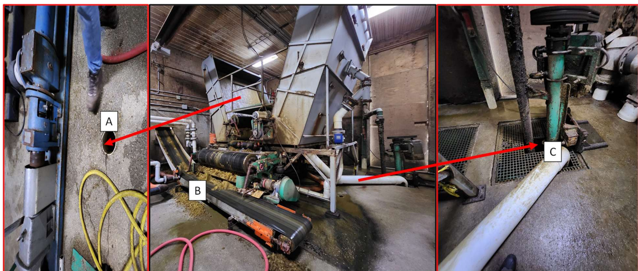
Figure 2. Slope screen and roller press. A) Liquid manure pre slope screen B) Solids post slope screen and roller press C) Liquid manure post slope screen and roller press.
