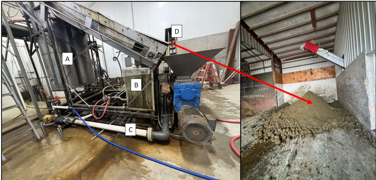
Figure 3. LWR slope screen and screw press. A) Liquid Manure pre LWR slope screen B) Liquid manure post LWR slope screen C) Liquid manure post screw press D) Final solids post LWR screw press
