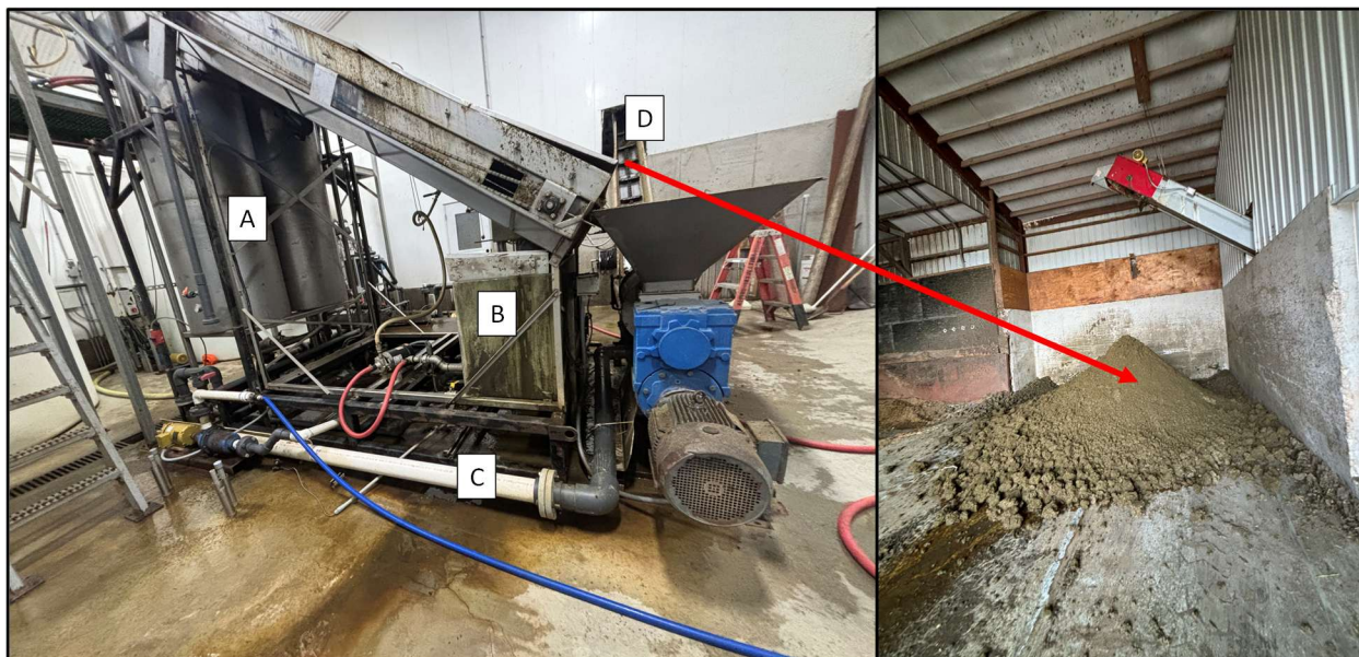
Figure 3. LWR “First Wave” slope screen and screw press. A) Liquid Manure pre LWR “First Wave” slope screen B) Liquid manure post LWR “First Wave” slope screen C) Liquid manure post screw press D) Final solids post LWR screw press.
