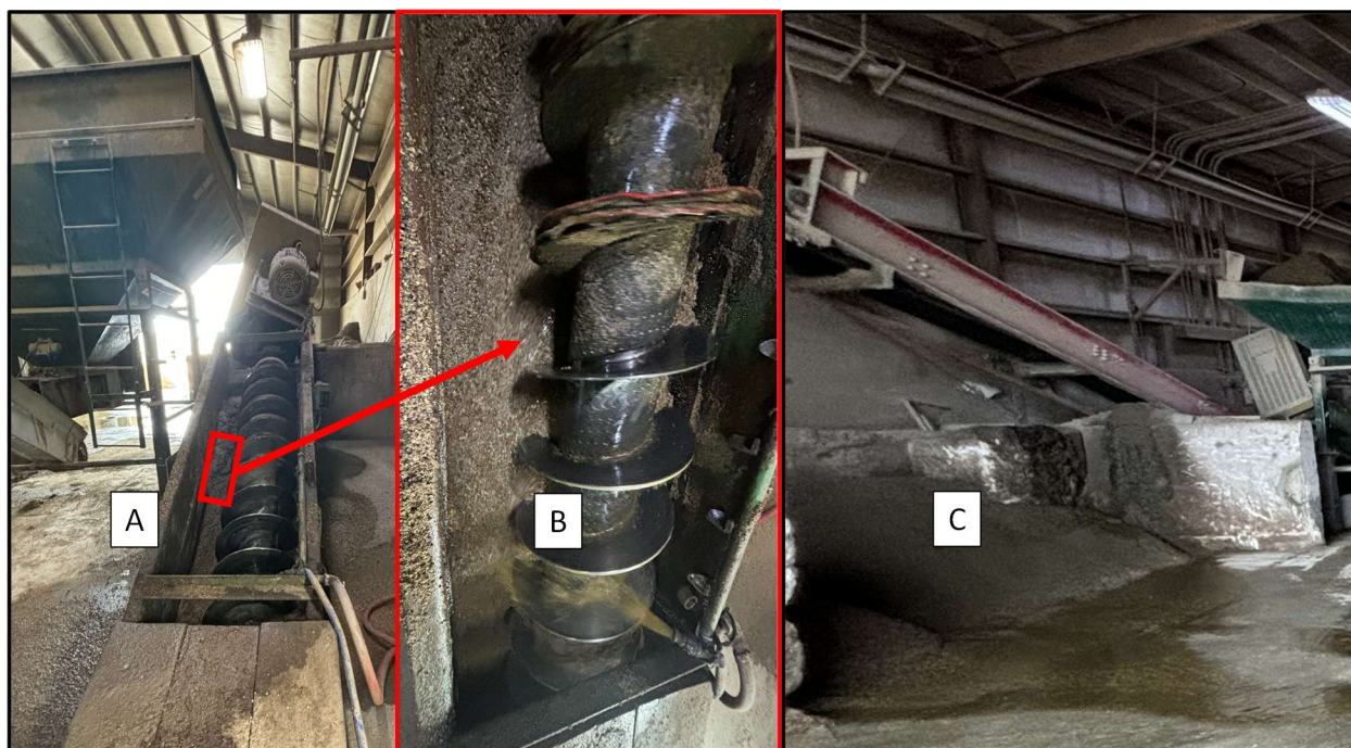
Figure 2. Sand Recovery System A) McLanahan system, B) close up of sand washing and recovery, and C) separated wet sand post recovery.
