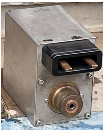
Figure 22. Plasma torch used by the prototype N2 Applied unit studied.
