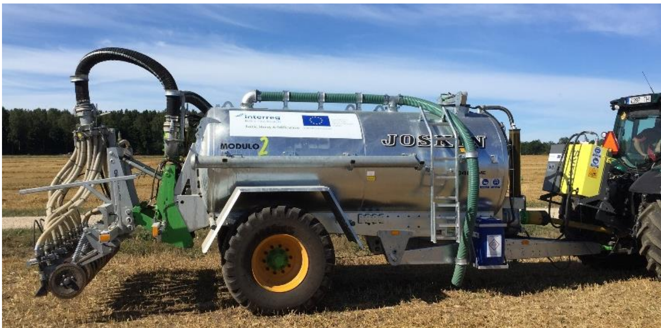
SyreN Light in use by an 8.000 m3 slurry tanker
