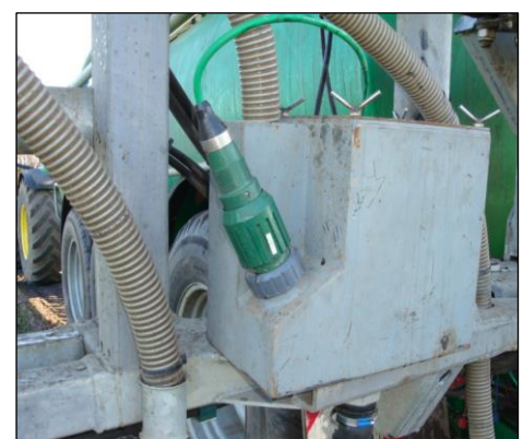
Slurry Sump with PH sensor
