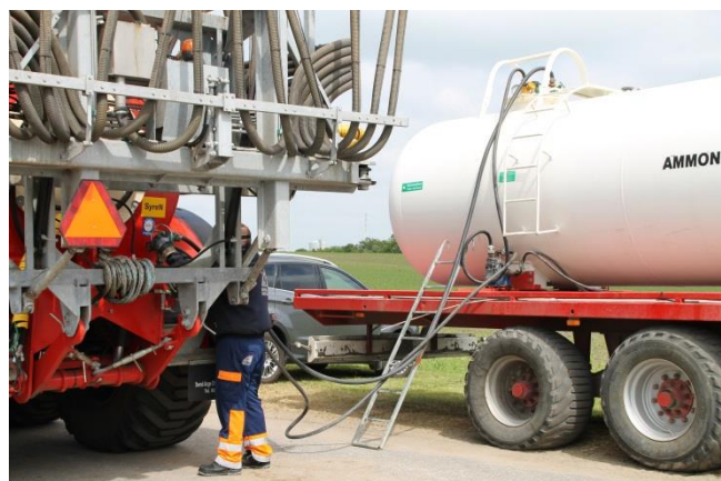
Filling of ammonia pressure tank
