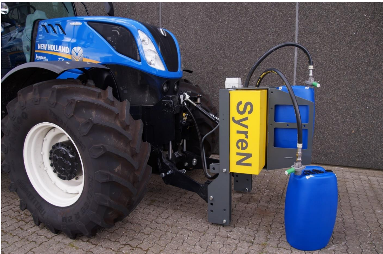
SyreN Light installed in the front hitch
