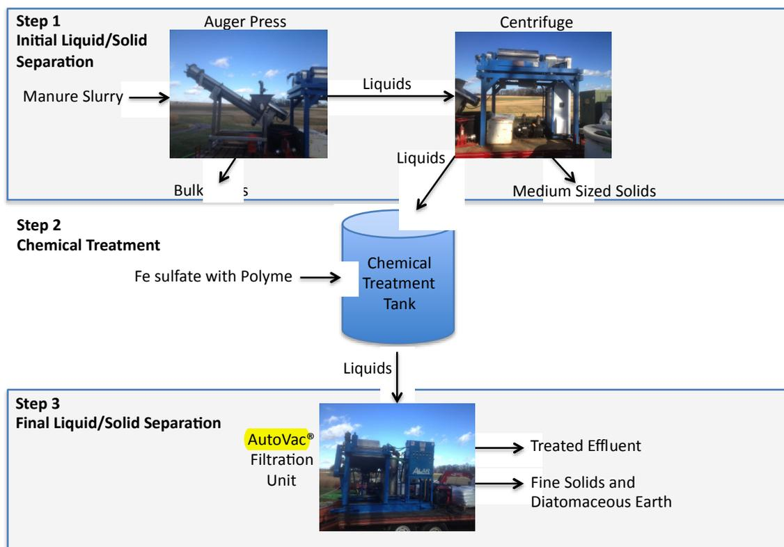
**Figure 3. The MAPHEX System, showing two-stage, liquid-solid separation step, chemical treatment, and final liquid-solid separation steps.**
