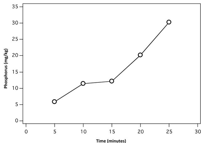
Figure 4. Phosphorus in effluent of AutoVac<sup>®</sup> when AMDR was incorporated into the filter pack.
