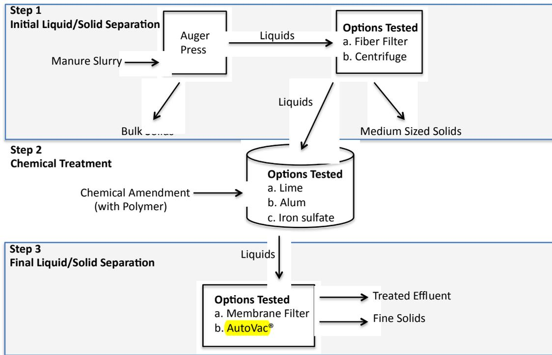
Figure 2. Flow chart showing options tested in designing MAPHEX system.
