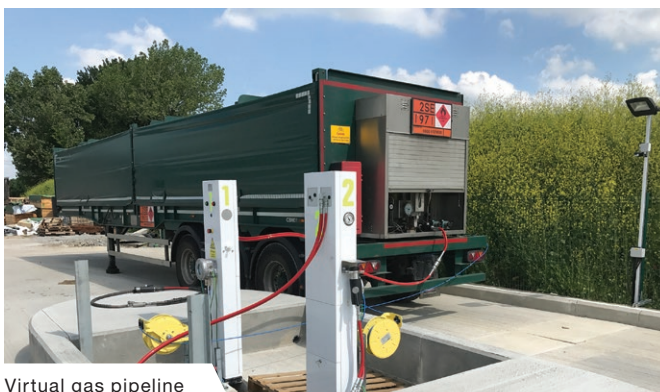
Virtual gas pipeline
